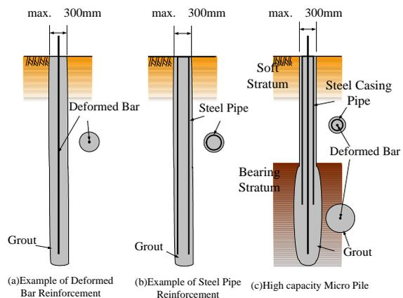
Fig-1.2 Structure of the Micropiles
