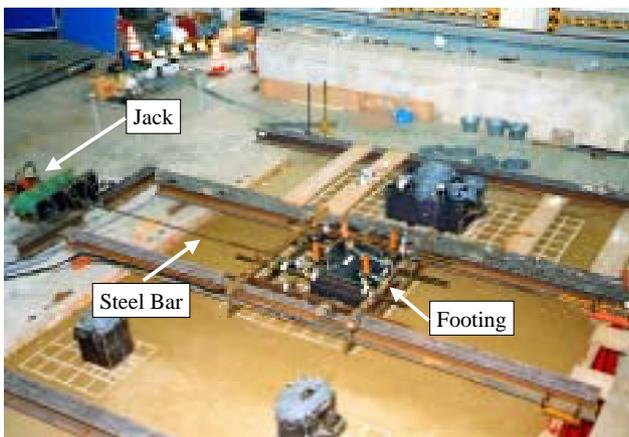
Photograph-2.1 Loading Test for Case 3
