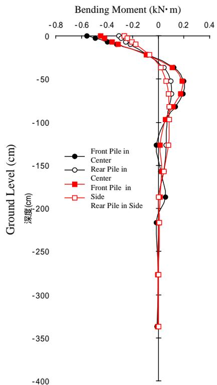
Fig-2.4 Bending Moment on Micropiles in Case 4
