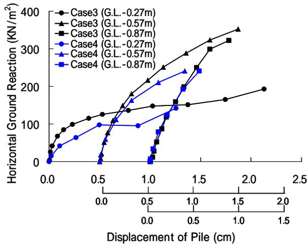
Fig-2.6 Curve of Horizontal Ground Reaction and Displacement
