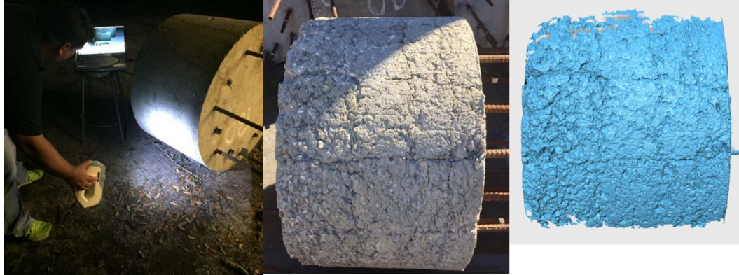
Figure 5: Scanning specimen (left), shaft photo (center), digital rendering (right).
