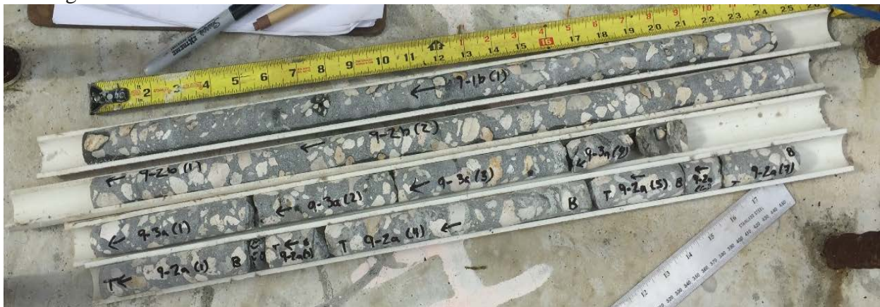
Figure 14: Cores extracted from Shaft 9-B50 (bottom two specimens extracted from the cover region)
