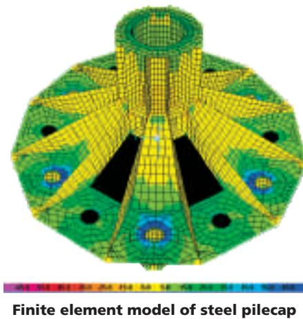
Finite element model of steel pilecap
